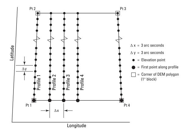
Figure 1-2. Structure of a 1-degree digital elevation model, arc second grid.
