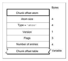
The chunk offset atom contains the following data elements.
