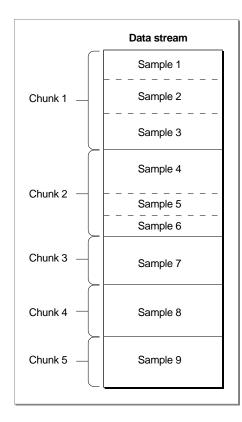
Chunks are a collection of data samples in a media that allow optimized data access. A chunk may contain one or more samples. Chunks in a media may have different sizes, and the individual samples within a chunk may have different sizes from one another.
