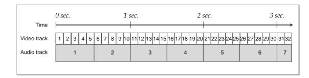
After the data has been interleaved on the disk, the movie data atom contains movie data in the order shown in Figure 1-46.
