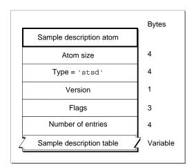
Figure 1-30 The layout of a sample description atom
