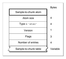
The sample-to-chunk atom contains the following data elements.
