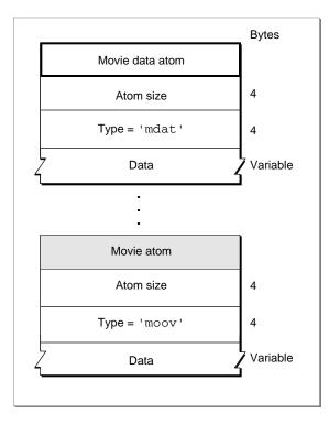
In file systems that support file name extensions, QuickTime file names typically have an extension of ".mov". On the Macintosh platform, QuickTime files have a file type of "MooV". On the Macintosh, the movie atom may be stored as a Macintosh resource using the Resource Manager. The resource has a type of 'moov'. All media data is stored in the data fork.
