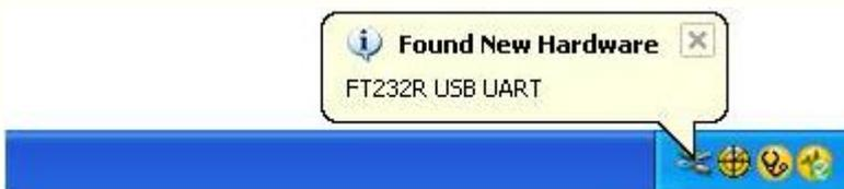
Most PC's will sound a tone that indicates a new USB device has been connected. Most Windows Vista and 7 systems will either include the FTDI device driver or are able to download it automatically from the network.
