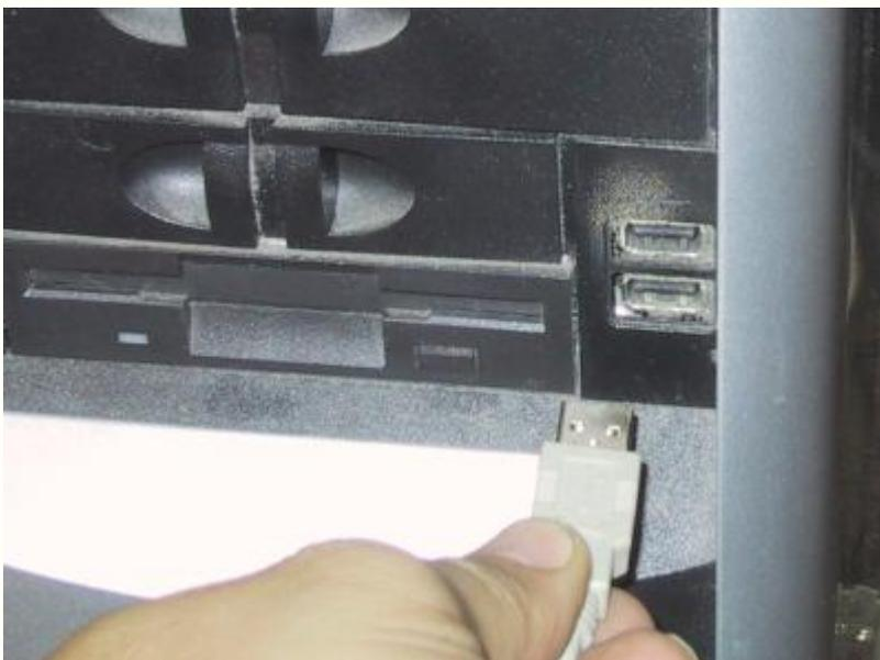
Locate the USB jack on your computer and plug the other end of the cable into it.
